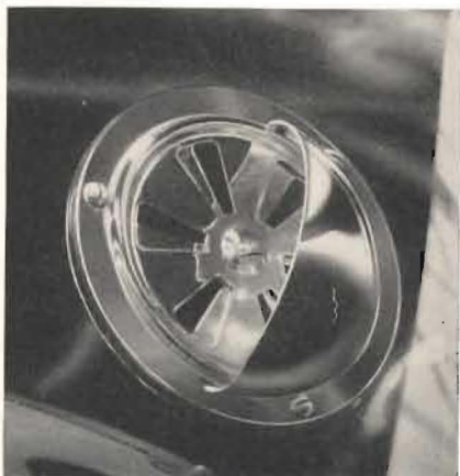
A ventilator shown in the half-open position.
