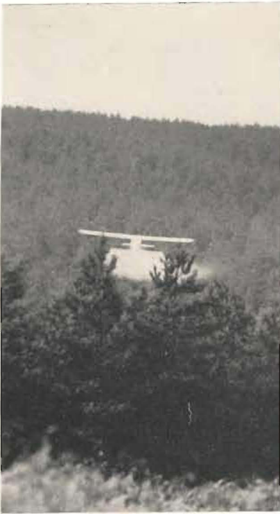
Down in the dell. One of the Auster Autocars follows the contours to obtain maximum penetration of spray through the pines.
